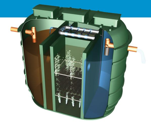
The FlowPath contains two stage primary settlement zones, designed to settle coarse and non-biological loadings.
